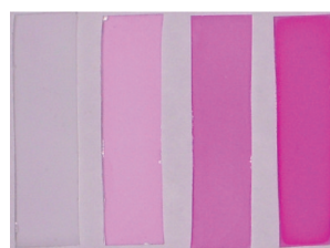
FIGURE 7. Photographs of the test strips with I ( 5.0 \times 10^{-4} M) for the detection of \text{Cu}^{2+} in aqueous solution with different concentrations. From left to right (M): 0, 1.0 \times 10^{-5} , 1.0 \times 10^{-4} , 1.0 \times 10^{-3} .
