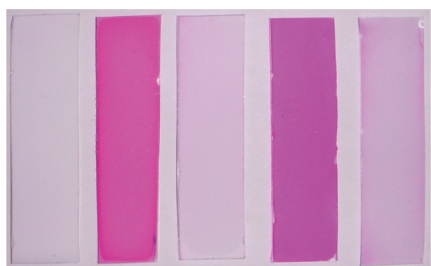
FIGURE 8. Photographs of the test strips with I ( 5.0 \times 10^{-4} M) + \text{Cu}^{2+} ( 1.0 \times 10^{-3} M) for the detection of \text{CN}^- in aqueous solution. From left to right: I , I + \text{Cu}^{2+} , I + \text{Cu}^{2+} + \text{CN}^- , I + \text{Cu}^{2+} + a mixture of anions ( \text{F}^- , \text{Cl}^- , \text{I}^- , \text{IO}_3^- , \text{SO}_4^{2-} , \text{NO}_2^- , \text{Br}^- , \text{H}_2\text{PO}_4^- , \text{HSO}_4^- , \text{ClO}_4^- , \text{SCN}^- ), I + \text{Cu}^{2+} + \text{CN}^- + the mixture of anions. The concentration of anions was 1.0 \times 10^{-2} M.
